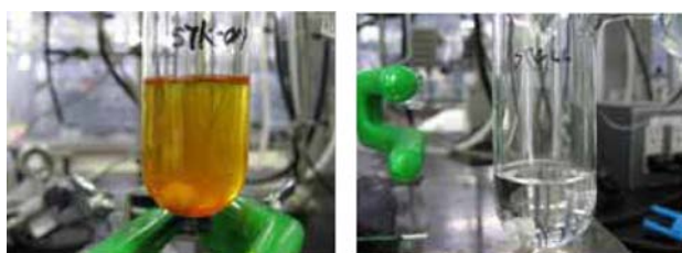
Figure 2. MAZ prepared with homogeneous 1 /MMAO/ \text{Ph}_3\text{CB}(\text{C}_6\text{F}_5)_4 (left) and with \text{SiO}_2 -supported 1 /MAO (right).
